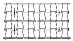
All welded selvage belts over 24 inches in width feature the resistance welding of every other connector rod to the flat strip on the 2nd opening in from each edge of the belt. On True 1/2" x 1/2" mesh belts this weld is on every 3rd connector rod.
