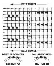
Proper sprocket location is essential for smooth belt operation. Sprocket teeth must always drive against the connector rods. Drive sprocket teeth should be in the odd numbered openings and tail sprocket teeth in the even numbered openings.
